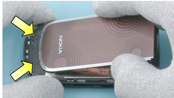
26) Use the guidings on the top side of the HINGE ASSY to attach the A-COVER WINDOW ASSY correctly.
