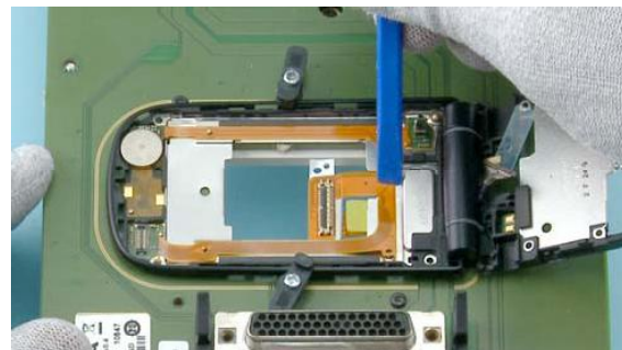
10) Use the SS-93 to attach the UI FLEX ASSY to the B-COVER.
