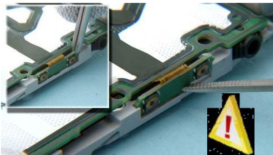
15) Lift up the VOLUME KEYS slightly with the tweezers. Then insert the tweezers in the gap as shown and carefully lever out the VOLUME KEYS.
