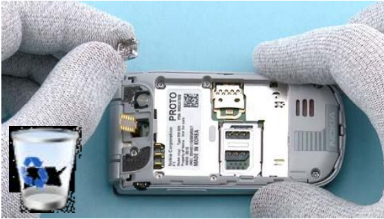
7) CAM. S.FLEX CLIP can be taken away. Do not use it again. Discard it.
