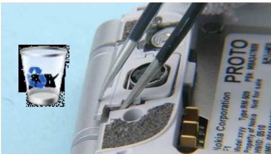
4) Remove the CAMERA FRAME ASSY with the tweezers. Do not use it again. Discard it.
