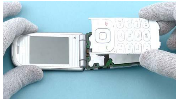
14) Fold open the phone. The KEYPAD can be removed.
