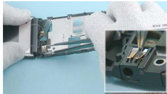
34) Place the DC jack with the tweezers.
