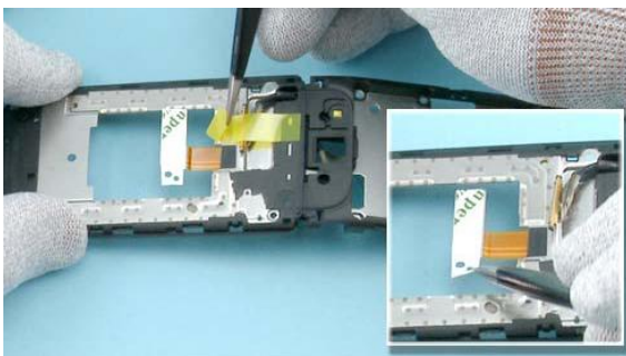
11) Use the tweezers to peel off the tape holding the MCX CABLE. Then remove the remaining protective film from the UI FLEX ASSY.
