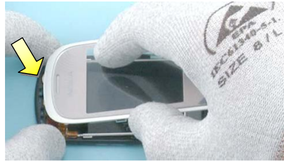
20) Attach first the top side of the B-COVER TRIM ASSY to the B-COVER.
