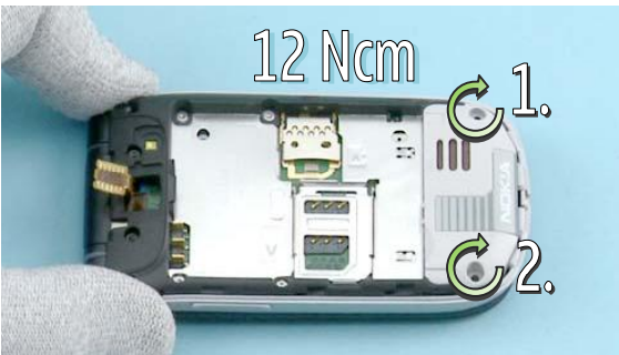
47) Tighten the two TORX + size 6 screws to the torque of 12 Ncm in the order shown.
