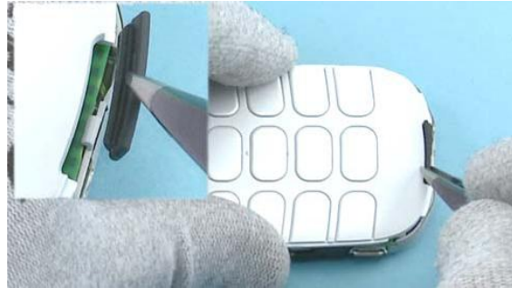
44) Place the stopper onto the engine board with the tweezers and fold the device.
