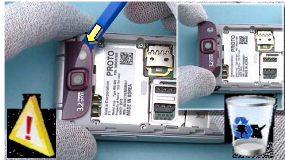
4) Lift up the CAMERA BEZEL ASSY with the SS-93. Be careful not to damage the CAMERA! Do not use the CAMERA BEZEL ASSY again. Discard it.
