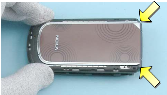
27) Also check with these guidings that the A-COVER WINDOW ASSY is correctly placed. Then press the A-COVER WINDOW ASSY firmly to activate the adhesive. Be careful not to damage the secondary display.
