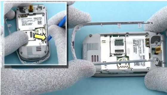
13) Also, detach the two clips on the other side. The C-COVER TRIM ASSY can now be removed.
