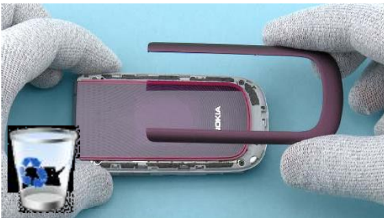
29) Remove the A-COVER ASSY. Do not use it again. Discard it.
