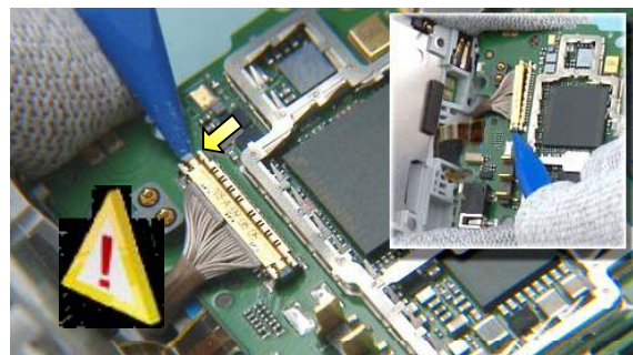
18) Disconnect the MCX CABLE from the UI FLEX ASSY using the sharp end of the SS-93. Be careful not to damage the connector or any nearby components!
