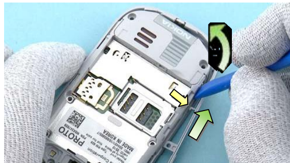
12) Slide the SS-93 along the side to release the shown clip.
