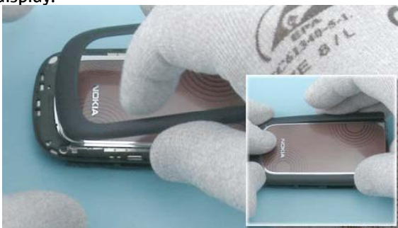
29) First attach the top side of the A-COVER ASSY. Then press the edges of the A-COVER ASSY firmly to attach the side clips correctly.
