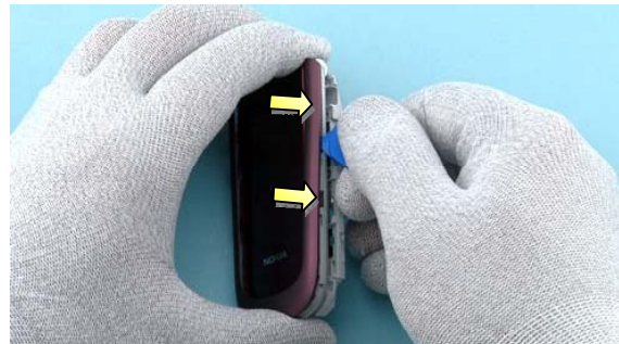
28) Then detach the two remaining clips on the other side.
