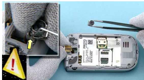
6) To remove the CAMERA MODULE, use the dental tool to bend the sides of the CAM S.FLEX CLIP holding the CAMERA MODULE. Be aware of the sharp point of the dental tool - be careful not to injure yourself! The CAMERA MODULE can be removed.
