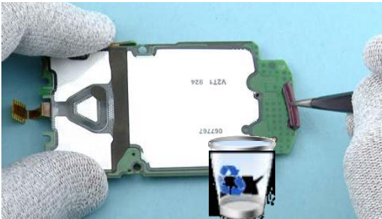
19) Remove the RUBBER STOPPER ASSY using the tweezers. Do not use it again. Discard it.
