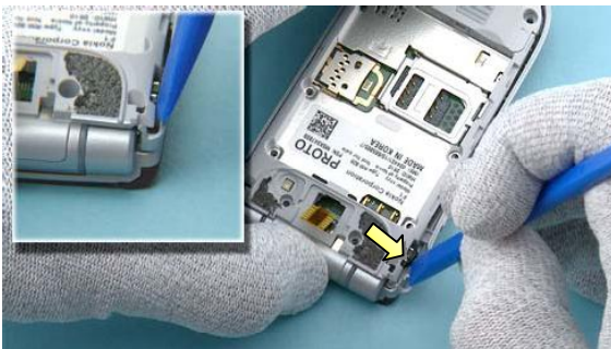
11) Start to detach the C-COVER TRIM ASSY by releasing the shown clip with the SS-93.
