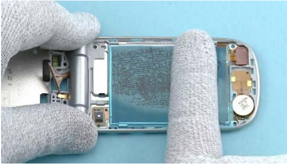
37) Protect the LCD with a protective film.
