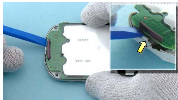
16) Use the SS-93 to release the clip holding the PWB.
