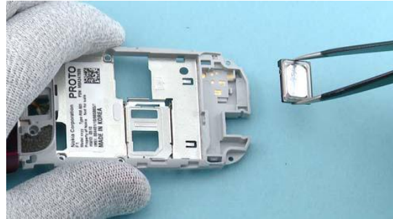
26) Remove the IHF SPEAKER with the tweezers.
