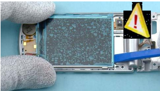
41) Carefully, place the SS-93 as shown and lift up the LCD. Be very careful not to break the LCD!
