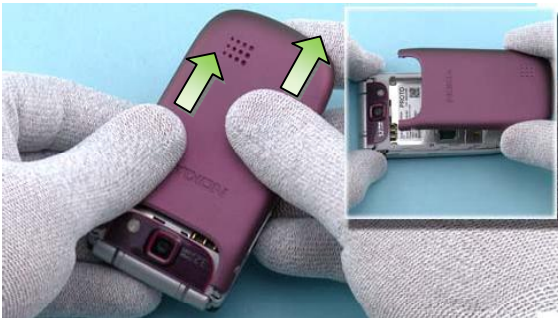
3) Detach and remove the D-COVER ASSY in the direction shown.
