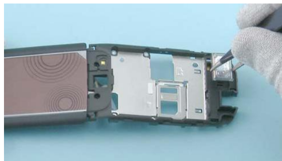
30) Insert the IHF SPEAKER into the slot shown with the tweezers.
