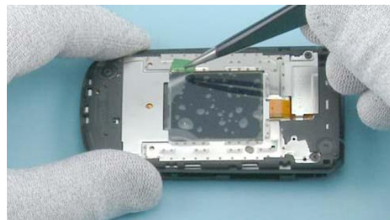
24) Remove the protective film from the secondary display.
