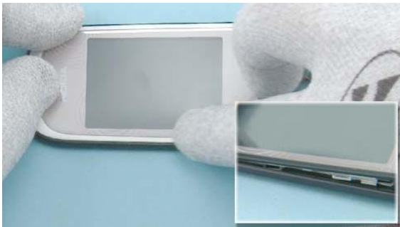
21) Press the edges of the B-COVER TRIM ASSY firmly to attach the side clips correctly.
