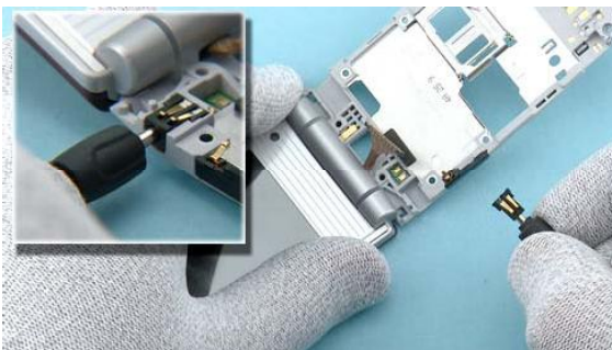
21) Lift up and remove the DC JACK with a DC plug.
