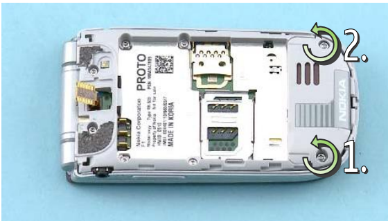
9) Unscrew the two TORX+ size 6 screws in the order shown. Note that these screws can be reused! Do not discard them.
