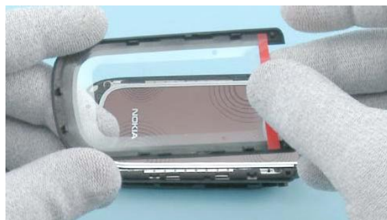
28) Remove the protective film from a new A-COVER ASSY.
